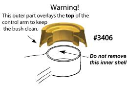
Place the upper vertical bushing #3406 in the metal shell first, this enables you to confirm that the inside edge of the bushing is not pinched at the top of the shell. Neglecting this step could cause the bushing to bind and or eventually tear.
