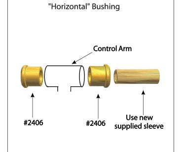
NOTE: Remember to remove any burrs from inside of the control arm to ensure proper operation.
